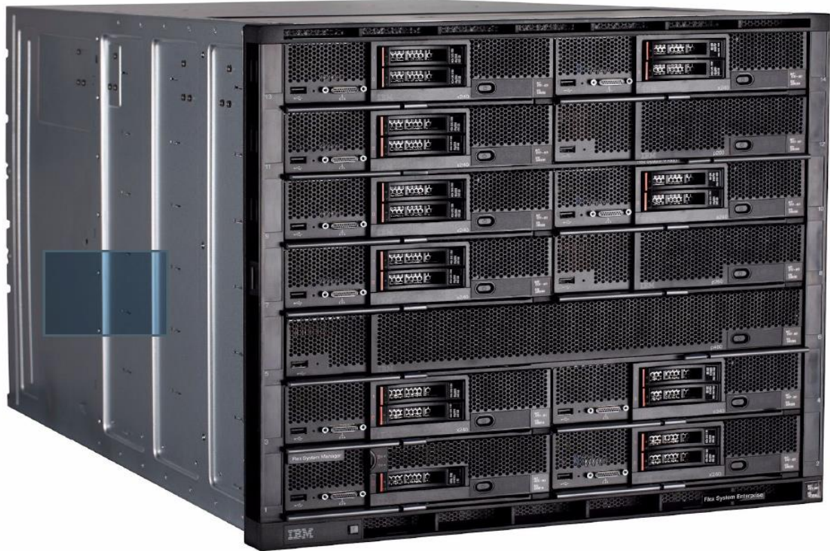
Figure 1-2 The IBM Flex System Enterprise Chassis
