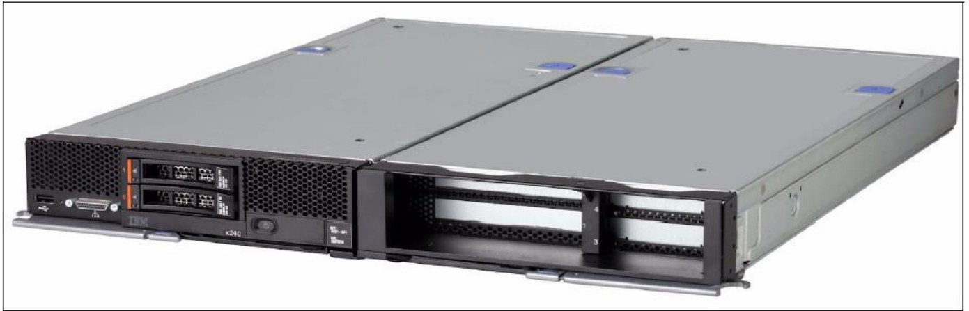
Figure 5-71 IBM Flex System PCIe Expansion Node attached to a compute node
